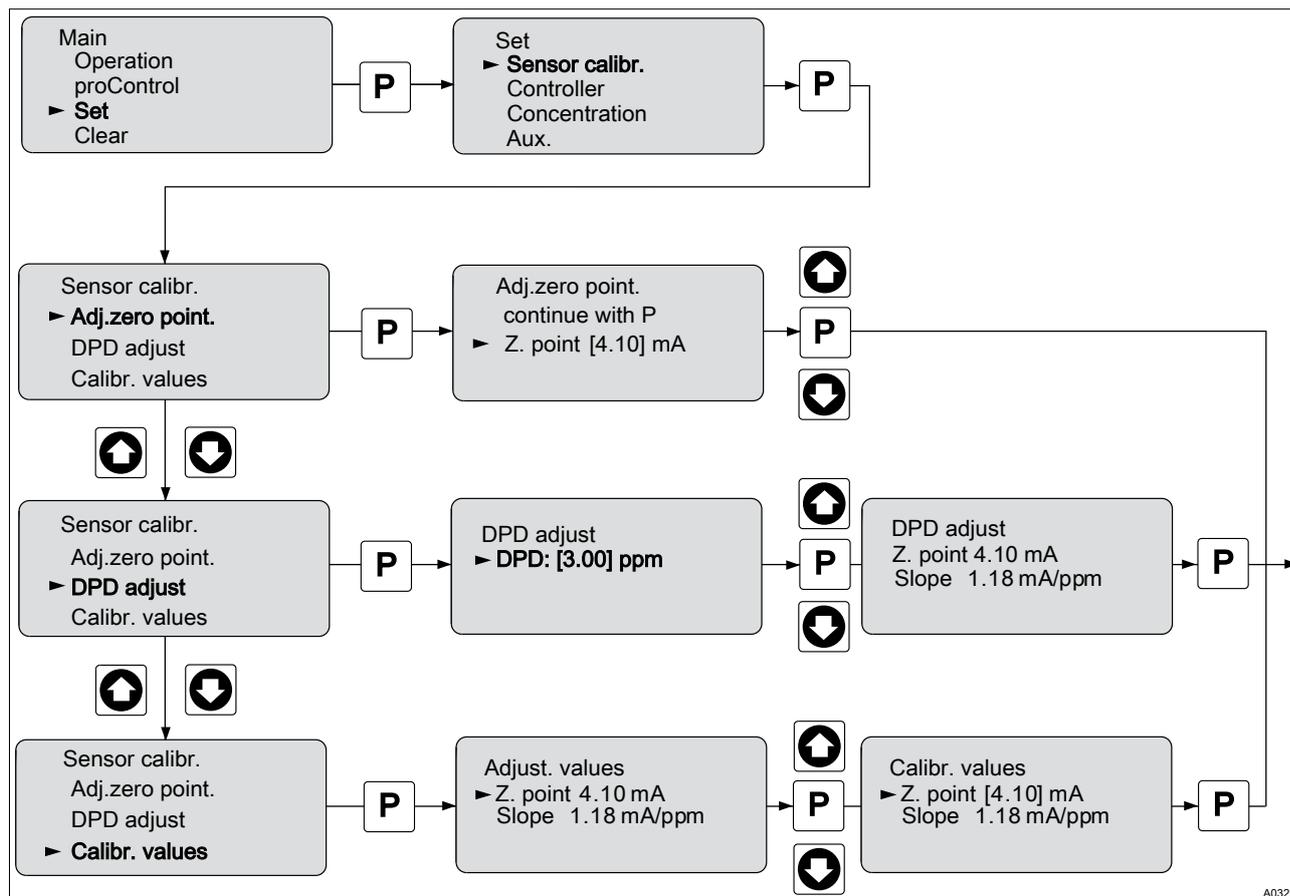
Fig. 26: Calibrating the sensor for chlorine
