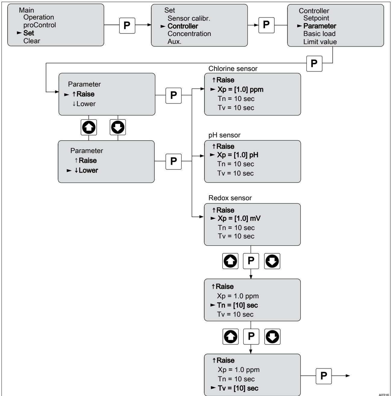
Fig. 20: Setting the control module delta®
