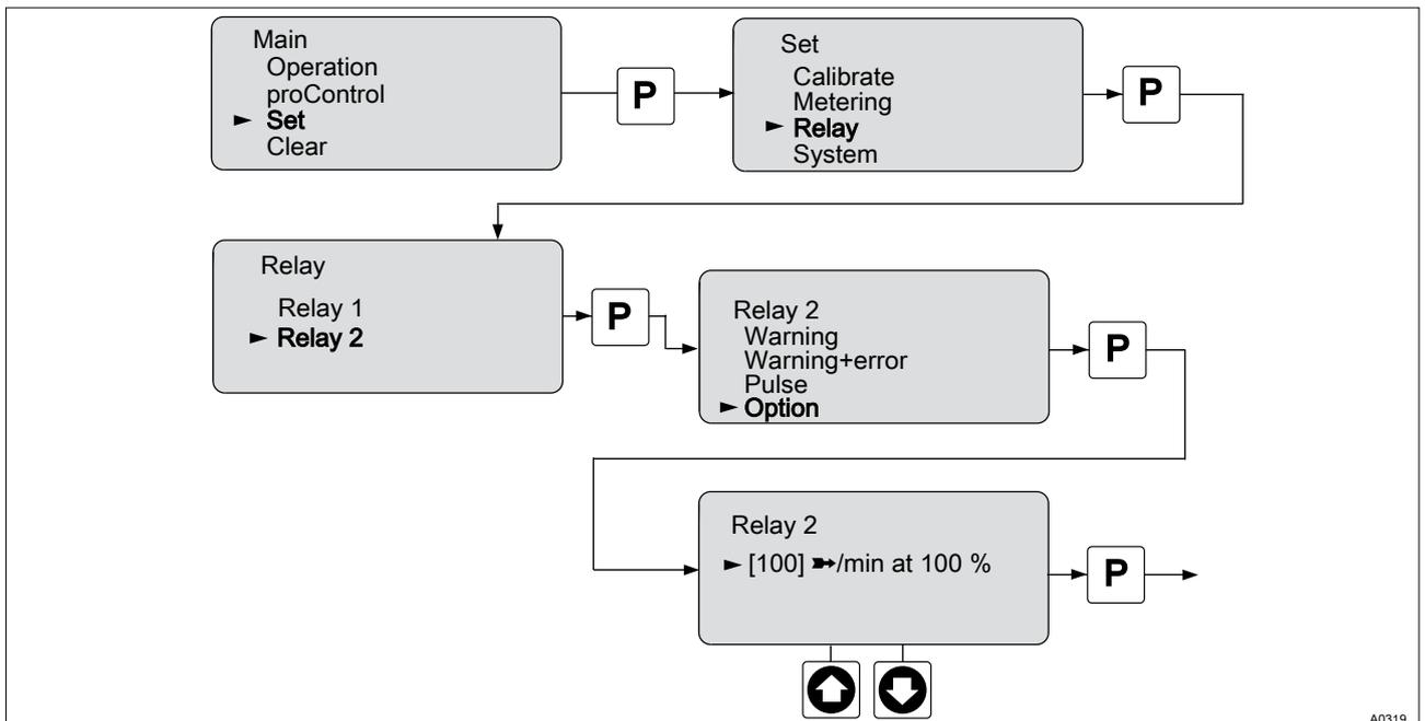
Fig. 23: Menu for adjusting the controller pulse of the second pump
