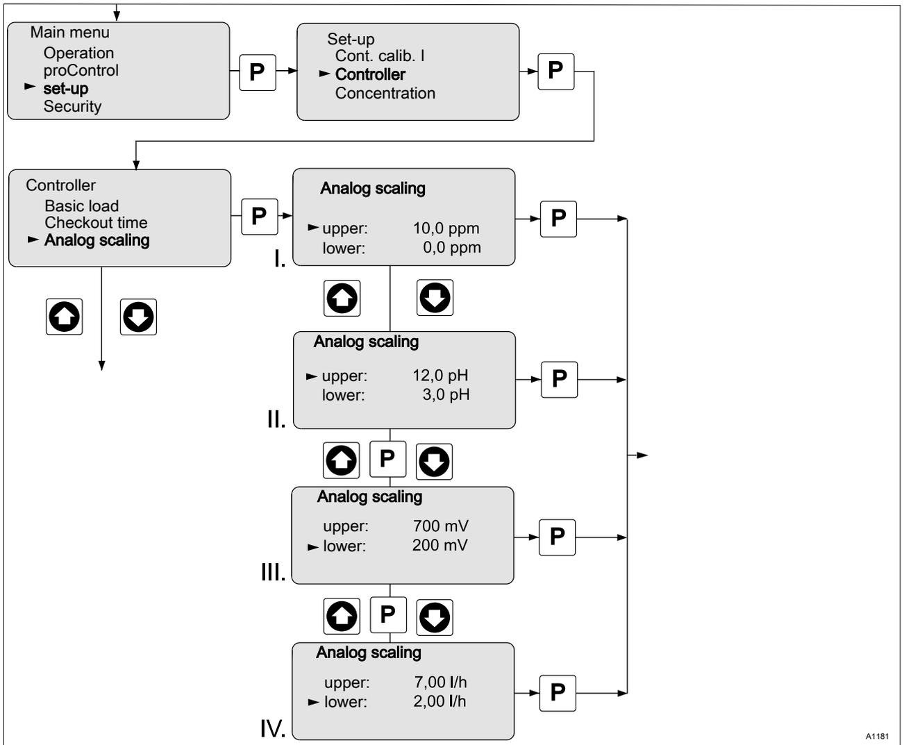
Fig. 25: Scaling the Output Value of the Analog Value
