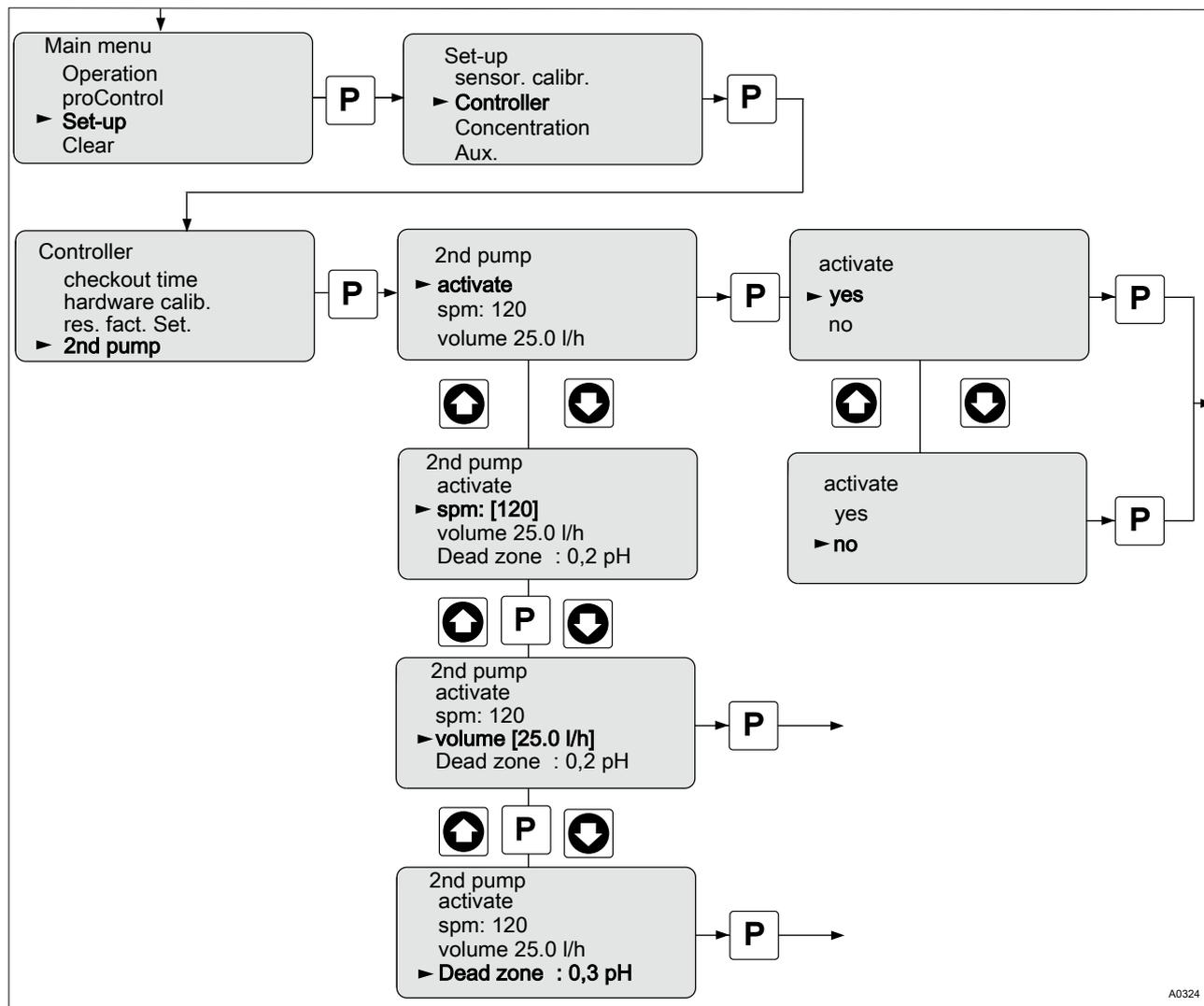
Fig. 22: Setting up "Two pump operation"
