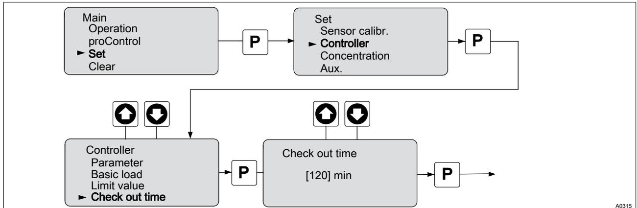
Fig. 19: Checkout time adjustment
