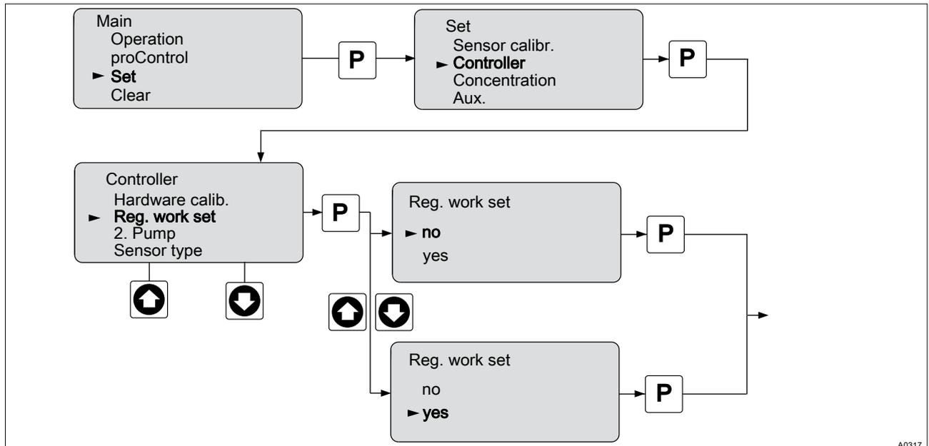
Fig. 21: Factory Settings of the control module delta®
