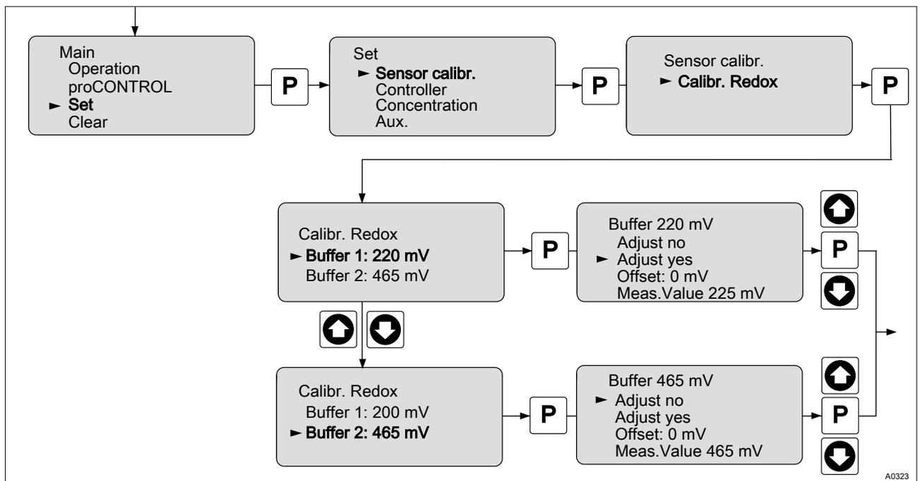
Fig. 28: Calibrating the sensor for Redox
