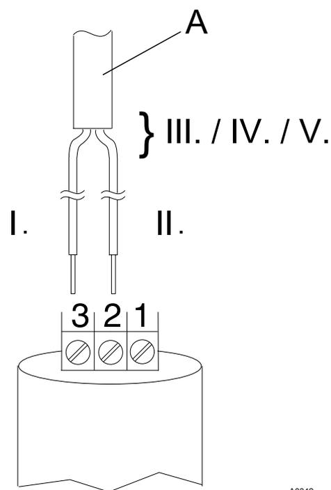
Fig. 4: Connection of the flow sensor
