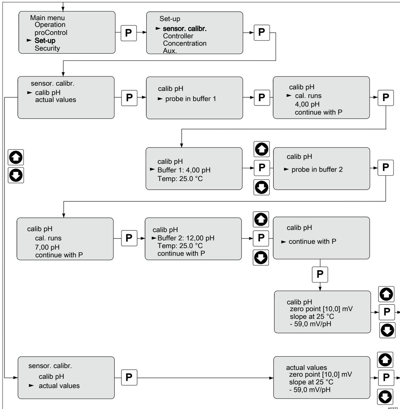
Fig. 27: Sensor pH calibration
