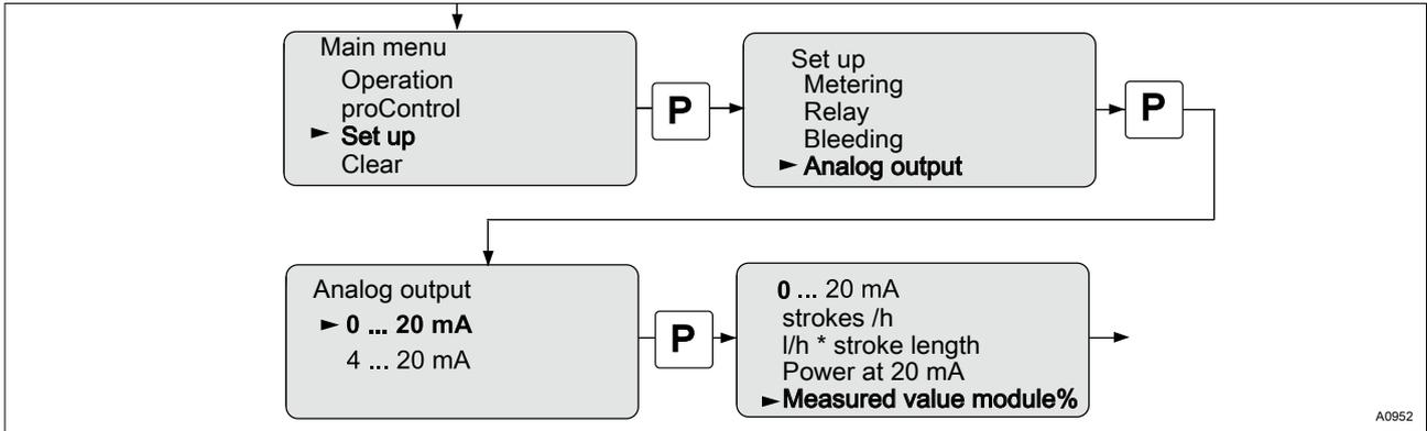
Fig. 24: Current output activation menu
