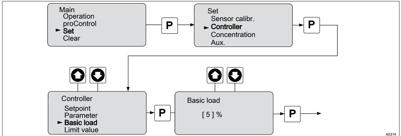
Fig. 17: Setting the basic load
