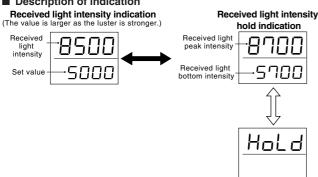
Selecting the displaying channel: While holding down the MODE button, press the UP or DOWN button.
