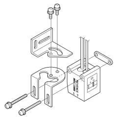
The sensor angle can be adjusted within  $90^{\circ}$  ( $\pm$   $45^{\circ}$ ). (Refer to the lower right of page 9.)
