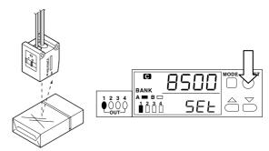
2 Place a target without a film onto the focus position of the beam spot emitted from the sensor. Then press the SET button once.
