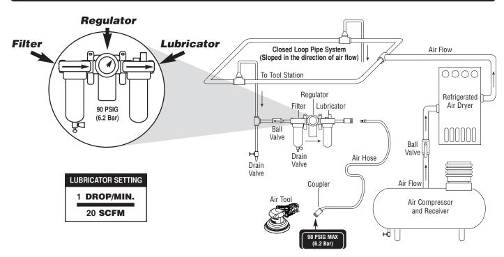
Dynabrade Air Power Tools are designed to operate at 90 PSIG (6.2 Bar/620 kPa) maximum air pressure at the tool inlet, when the tool is running. Use recommended regulator to control air pressure. Ideally the air supply should be free of moisture.
