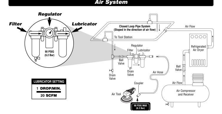
Dynabrade Air Power Tools are designed to operate at 90 PSIG (6.2 Bar/620 kPa) maximum air pressure at the tool inlet, when the tool is running. Use recommended regulator to control air pressure.  Ideally the air supply should be free of moisture. To facilitate removing moisture from air supply, the installation of a refrigerated air dryer after the compressor and the use of drain valves at each tool station is recommended.
