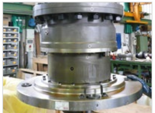
Shear pin type gear coupling
