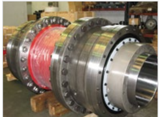
Dredger gear coupling
