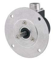
The optional SPY adapter is made of all aluminum construction and allows the Model 725 encoder to replace DC tachometer technology. The SPY adapter is mechanically interchangeable with any SPY tach generator.
