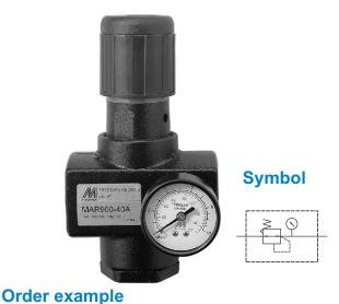
• MAR900 reducing the system pressure to a desired level and maintain it at a constant level despite change in inlet pressure and changes in downsteam flow requirements.
