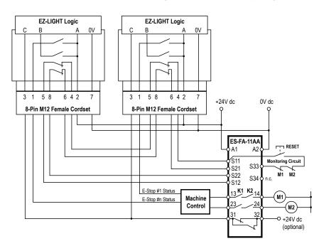
Note: Refer to the ES-FA-11AA E-Stop Safety Module datasheet (p/n 60606) for complete safety module installation information.
