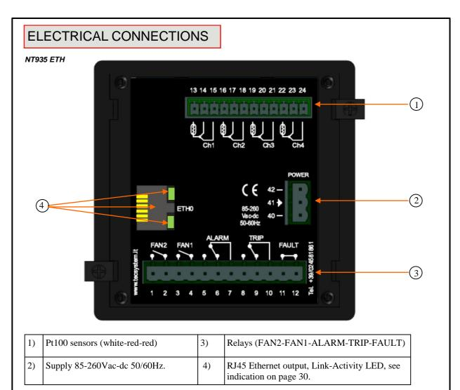
Note: relay contact image in non-alarm condition, with the exception of the FAULT relay that opens: contact 11-12 open (NO) contacts 11-12 closed (NC) fault condition identification. Read the Alarms and Ventilation paragraph on page 12 and see the opening of the fault contact.
